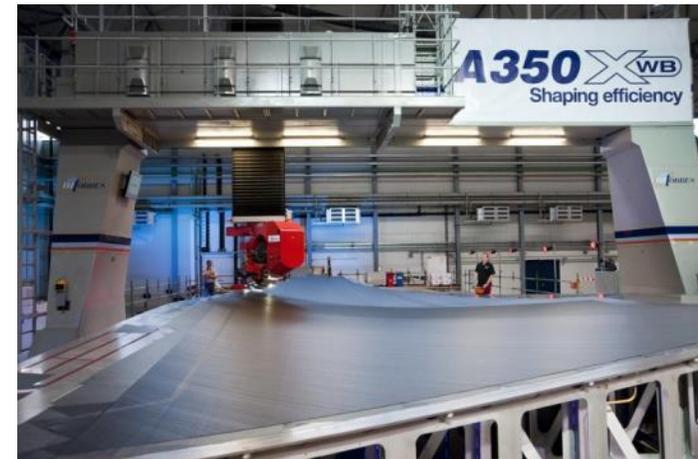
Tape laying for large scale CFRP parts
