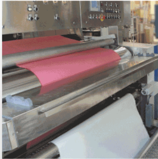
Easy-change Mini-pressure rollers with different surfaces and pressure adjustment system
