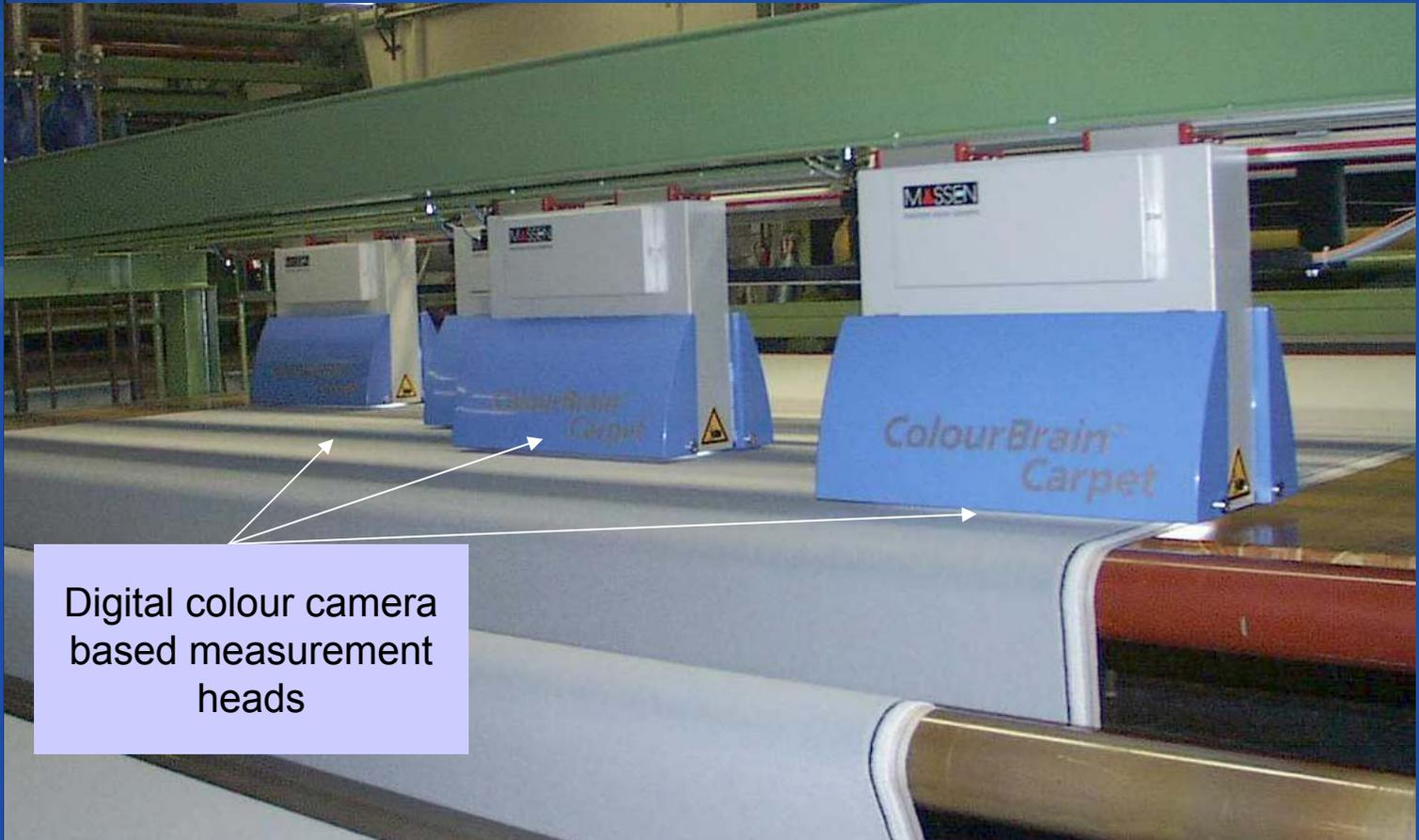
Digital colour camera based measurement heads
